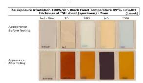
Very little color change after Xenon testing. This stability opens the door for choice of colorants to be used in cast systems with little change over long term UV exposure
